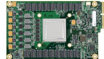
Figure 3. TPU Printed Circuit Board. It can be inserted in the slot for an SATA disk in a server, but the card uses PCIe Gen3 x16.
